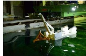
Fig. 8 Model test in waves for crane barge
